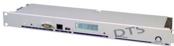
E.g. DTS 4135.timeserver; high accurate multi purpose timeserver
