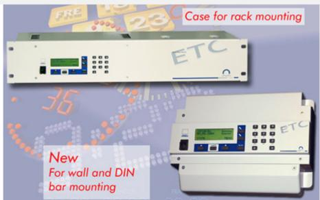
The EuroTime Center ETC operates conventional clock systems with impulse controlled slave clocks as well as modern, self-setting MOBALine installations. Easy and intuitive operation control due to ETC's intelligible user interface. ETC's power relays control light, heating, signalling-bells and other devices by weekly periodic and/or date related programs. Absolute precision of ETC's internal clock can be achieved by synchronization to an external time-reference such DCF77 or GPS.
