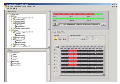
Optional software running in the familiar WINDOWS environment enable even complex switching and signalling programs to be produced in a clear way and then loaded in the master clock via the serial interface.
